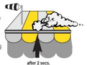
All manual or automatic commands are inhibited as long as the wind speed is higher than the adjusted threshold.
