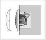
Connect the wires to the terminals of the connecting bracket in accordance with the terminal layout (chapter 2.2).
