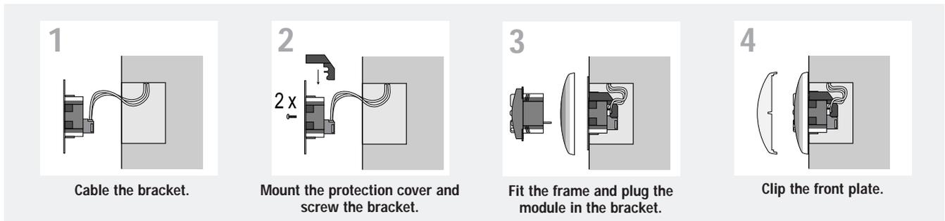
Do not forget to mount the protection cover to separate the cables for the BUS line and the cables for the power.
